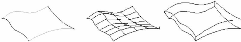
**Figure 27. Thickening surfaces into solids.**
